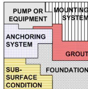
Consider all of the components and how they work together to create a monolithic structure when designing for optimum equipment performance
