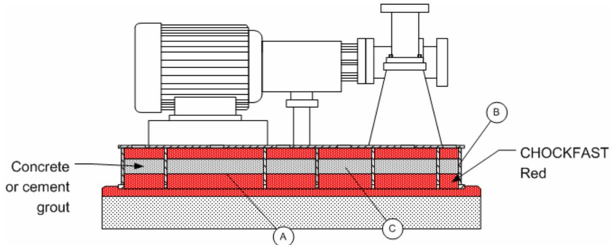
C - Concrete requires a minimum of 28 days to cure and lower its water content enough so the epoxy grout poured on top of it will bond. If epoxy grout is poured on top of the concrete too soon water will dissolve the epoxy hardener molecules at the bond line
